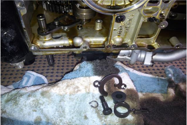
I then used a short socket extension bar in that hole in the selector drum to rotate the entire drum clockwise so I could disengage the selector quadrant:
