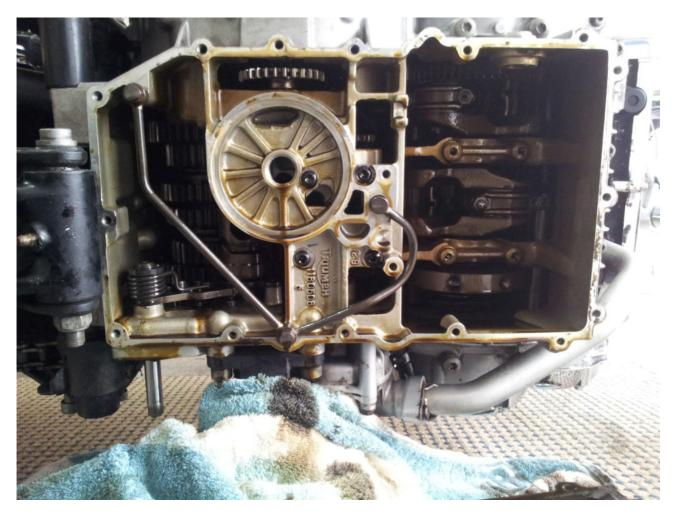
Next you need to remove that oil pipe, being careful not to lose the two copper washers under the banjo bolts. I used cable ties to keep them all together, like so:
