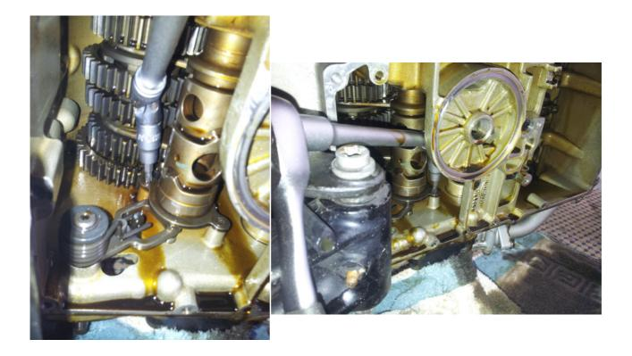
Next remove the retaining plate (b) by holding the right side of the plate and rotating it clockwise while pulling it back and toward you, like so:
