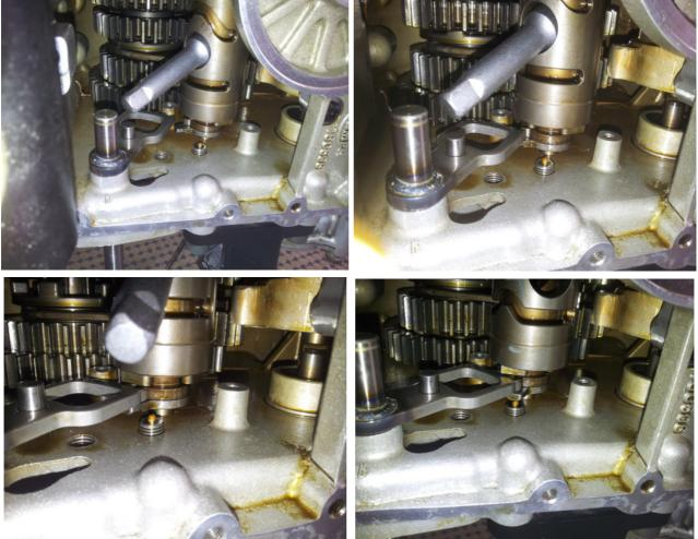
You need to end up with the middle tooth of the drum in the middle hole of the quadrant -
