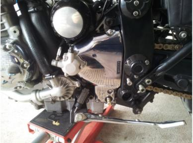
Fill the engine with oil, don't forget this! I filled to halfway up the sightglass. After first start you will need to top this up as some oil is taken up in the rocker cover. Don't forget!
